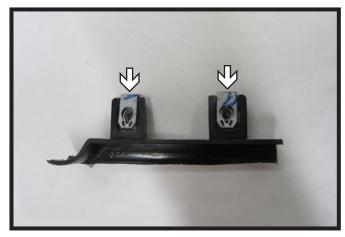
24. **Hybrid (4xe) Models**: Remove clips from the pedestrian alert bracket and set aside to be reinstalled later.
