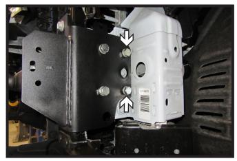
22. Install two (2) 1/2" x 1-1/2" bolts with lock washers and whiz nuts back holes. Do this on both sides of the vehicle. Tighten all bolts at this time.
