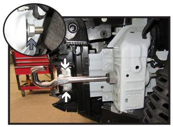
Using a 16MM socket, remove the two (2) bolts (white) from the tow hook. Then using a large crescent wrench, remove the nut (gray) from the back of the tow hook (inset). Remove tow hook and set aside to be reinstalled later. Do this on both sides of the vehicle.
