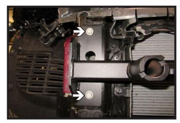
18. Hold baseplate into place on the vehicle frame and start the existing bolt in the top hole. Do this on both sides of the vehicle. Note: Ensure all holes line up before tightening bolts.
