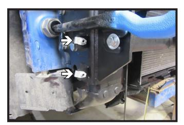
25. **Hybrid (4xe) Models**: Install clips from pedestrian alert bracket onto the tabs on the passenger side of the baseplate.
