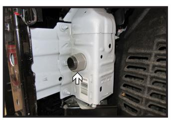
16. Using an extra large crescent wrench, remove the nut from the driver side of the vehicle. Slide tube back and out of the way to be reinstalled later.
