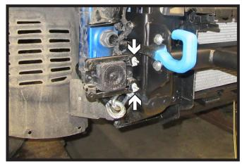
26. **Hybrid (4xe) Models**: Reinstall the pedestrian alert system onto the bracket on the passenger side of the vehicle using the existing bolts and hardware.
