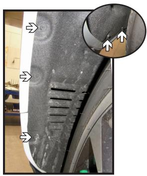
4. Using an 8MM socket, remove the five (5) bolts from along the edge of wheel well. Do this on both sides of the vehicle.
