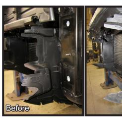
14. Using a utility knife, cut and remove the area from plastic shroud as shown. Do this on both sides of the vehicle.
