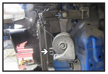
12. Unclip horn from the bracket (white). Then using a 10MM socket, remove the one (1) bolt (gray). Place the horn out of the way during baseplate installation, it will be reinstalled later. Do this on both sides of the vehicle.
