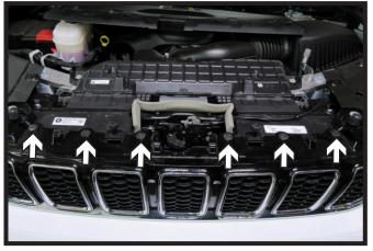
Using a T40 Torx, remove the six (6) bolts from the top of the fascia.
