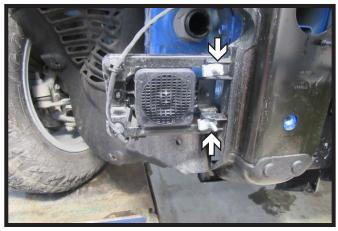
11. Hybrid (4xe) Models: Using a 10MM socket, remove the two (2) bolts from the backside of the pedestrian alert system. Remove alert system and set aside to be reinstalled later.
