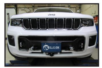
29a. **Non-Hybrid (4xe) Models**: Hold the fascia as close to its original position, mark and trim the fascia around the convenience links and attachment tabs. Reinstall the fascia, fascia cover, belly pan and reconnect all electrical connections.
