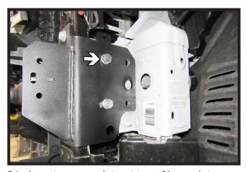
21. Insert spacer plate at top of baseplate between the frame and baseplate with the slotted end facing downward. Once spacer plate is in position insert 1/2" x 1-1/2" bolt with lock washer and whiz nut into top front hole.
