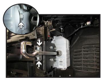
23. Reinstall tube with nut on the driver side of the vehicle. Then reinstall tow hooks on each side of the vehicle using two (2) 3/8" bolts with lock washers, flat washers, and a nylon lock nut for the top bolt and a nut plate for the bottom bolt. Reinstall existing nut on back of each tow hook (inset).
