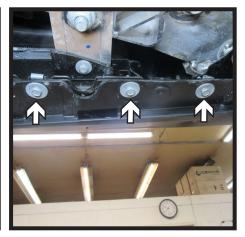
7b. Hybrid (4xe) Models: Using a 10MM socket, remove the nine (9) bolts from the underside of the vehicle. There are three (3) on each side and three (3) in the middle.
