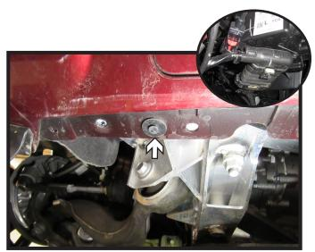
8a. Non-Hybrid (4xe) Models: Let belly pan hang and remove one (1) push pin from each side of the vehicle. Remove fascia, disconnecting all electrical (inset), and set aside and to be reinstalled later.
