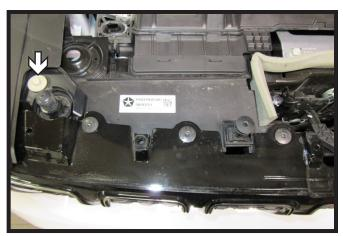
Using a 10MM socket, remove the one (1) bolt from the top of the fascia. Do this on both sides of the vehicle.
