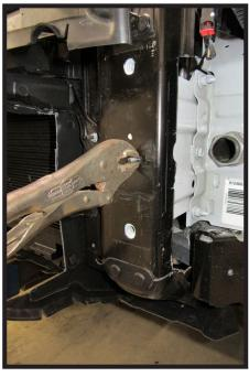
15. Using vice grip pliers, shake bolt to loosen. Then using a hammer, pound out bolt and remove. Do this on both sides of vehicle.
